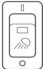
(2) Rear working light switch Rear working light switch
