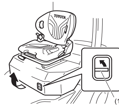
(1) Engine hood lock release lever
